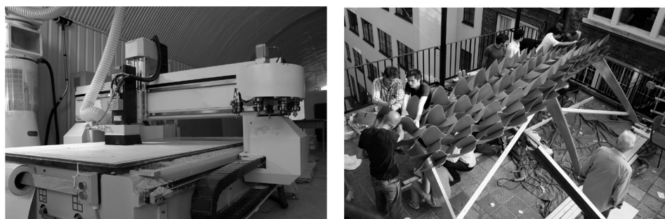
Fig. 2 CNC cutting of the components and assembly of EmTech Canopy 2009 at the Architectural Association in London.
